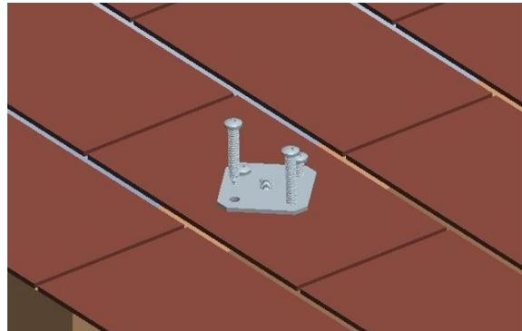
2. Attach the base to the roof by placing screws in and tightening them.
