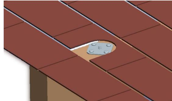
3. Properly cut the shingle by using the flashing template and a roof-cutting blade.
