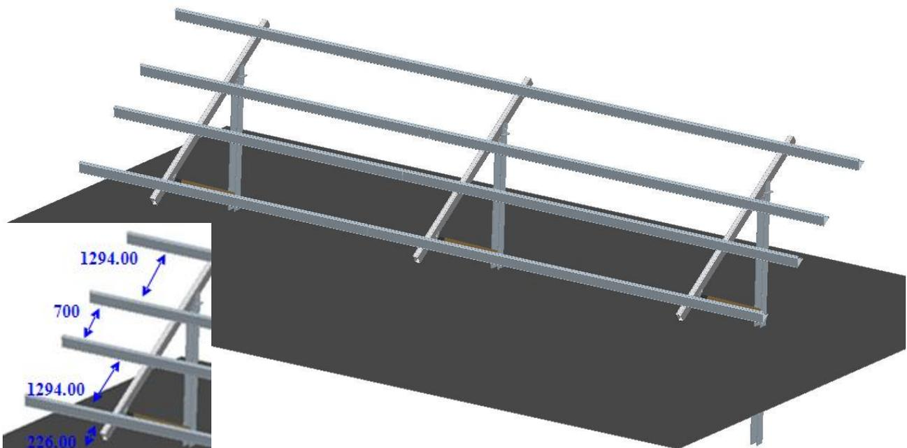
10. Fasten the other three purlins using the same steps listed above. Distances between the purlins are shown in the picture above. (Distances are measured from the center of the purlins)
