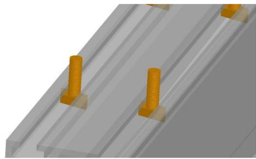
7. Turn four prismatic bolts into the groove of the girder.
