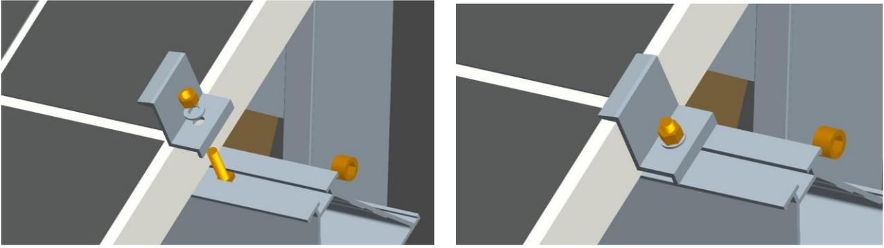
11. Insert prismatic bolts into the groove of the purlin and rotate to fix it into the groove. Fasten the solar panel with the end clamp and prismatic bolts.
