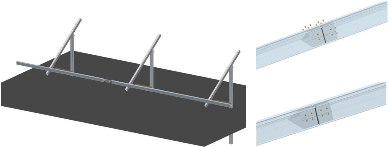
9. A splice can be used to expand this mounting system. First, insert the splice into one side of the purlin and secure it in place with bolts. Then loosely attach the second purlin onto the girder. Connect the two purlins together and secure them with bolts. A 10mm gap should remain between the two purlins.
