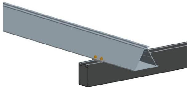
8. Fasten the purlin onto the girder with prismatic bolts.
