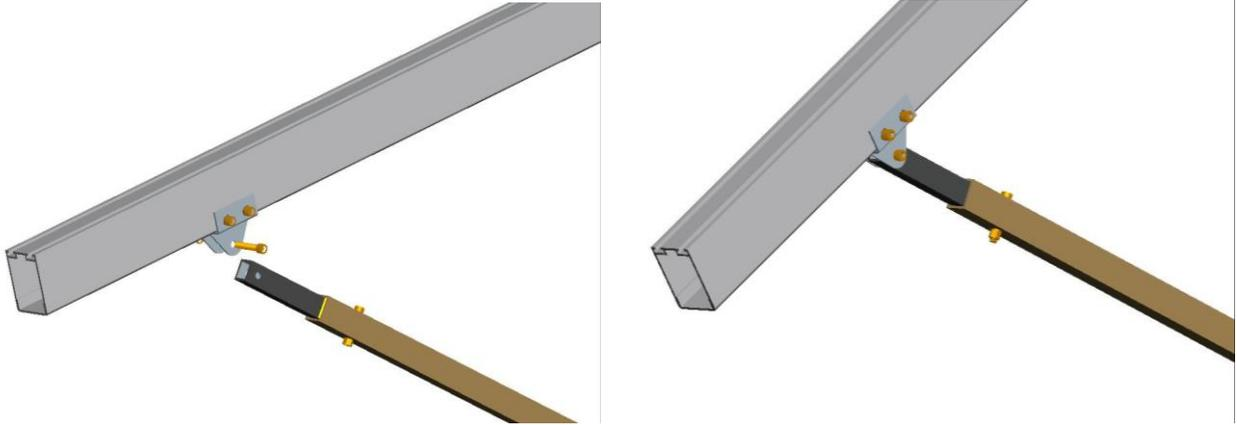
5. Insert the small strut into the large strut and fasten the other side of the small strut onto the strut console. Choose the mark showing the desired angle and insert a bolt into the hole on the big strut, then fasten it. There are five marks on the small strut indicating the different angles: 15°, 20°, 25°, 30° and 35°. Choose the right angle that optimizes your system.
