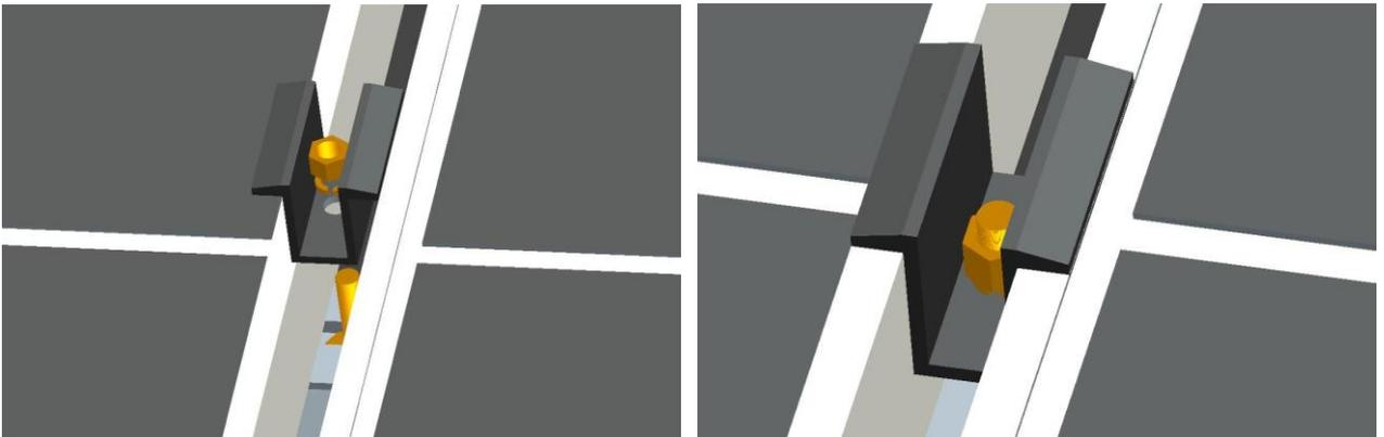
12. Insert prismatic bolts into the groove of the purlin and place it between two solar panels. Rotate to get it stuck in the groove. Fasten the solar panels by using a mid clamp.
