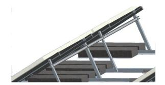
1, Place the first row in a line, and then put the east-west connect beam on the tilt leg, screw the bolts to fasten the east and west triangle systems.
