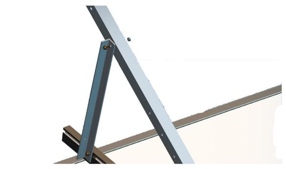
8, Screw the bolt to fasten the bottom beam and the tilt leg. There are four holes (hole 2, hole 3, hole 4, hole 5) to choose which can be used to adjusted the tilt-angle to 15°, 20°, 25° or 30°. (Note: choose the best triangle to optimize you PV system, please check the last page)
