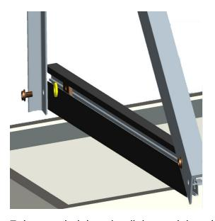
7, Insert a bolt into the tilt leg and though a gasket on the other side before screwing in the nut.
